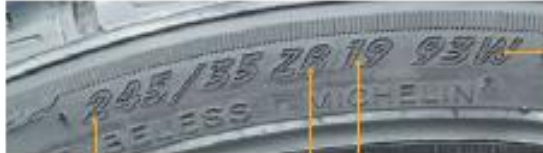
Section width and aspect Ratio (Example : 245/35) R = Radial tire Rim diameter (Example : 19) Load index & Speed index (Example : 93W)
