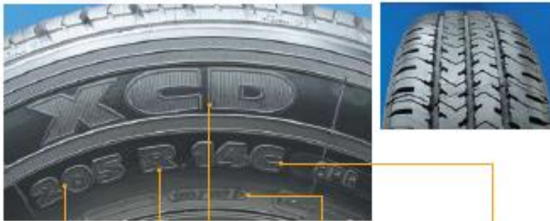
Section width (Example : 205) R = Radial tire Tread tire pattern (Example : XCD) Load index & Speed index (Example : 109/107P) Rim diameter (Example : 14) C=Camionette
