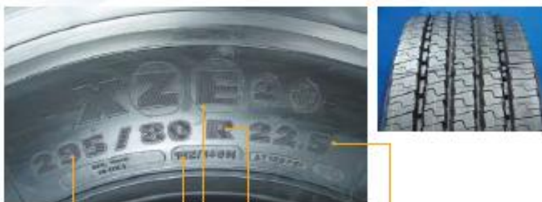
Section width and aspect Ratio (Example : 295/80) R = Radial tire Tread tire pattern (Example: XZE2+) Load index & Speed index (Example : 152/148M) Rim diameter (Example : 22.5)
